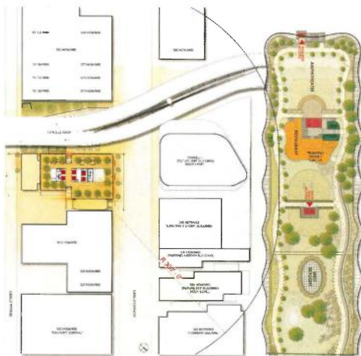
Figure 1. Location of the proposed 555 Howard Street tower (on the left) relative to Transbay Park. Areas within 300 feet of the 555 Howard Street tower are indicated by the dashed line. Note the proposed 806-foot tower between 555 Howard Street and the Park (labeled “Parcel F”). The other intervening buildings (at 530 and 540 Howard Street) are shorter than the proposed elevation of Transbay Park and do not obstruct the 555 Howard Street tower from the Park.
